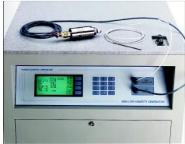
The main panel has easy access to the keypad, function keys, and test temperature and test pressure connectors.
